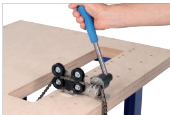
Cut chain to length push out the link rivet completely readjust at set screw if necessary
