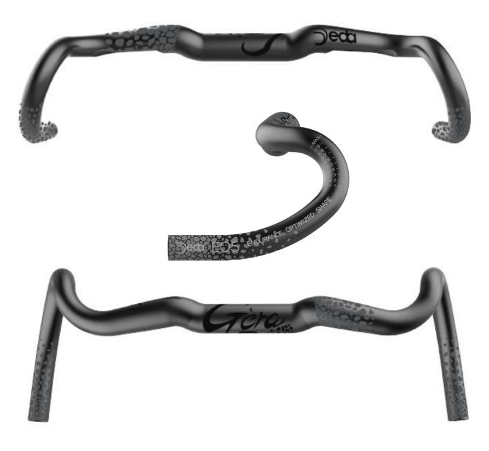
**SHAPE**: EOS (ENDURANCE OPTIMIZED SHAPE) MATERIAL: 6061 ALUMINUM DOUBLE BUTTED Ø HANDLEBAR: 31,7 MM REACH: 55 MM **DROP**: 100 MM **FLARE:** 24° **OUTSWEEP**: 3° **RISE**: 10° / 10 MM BACK SWEEP: 12° / 12MM **DOWNSWEEP:** 5° **WIDTH**: 42 – 44 – 46 – 48 CM (OUTSIDE-TO-OUTSIDE AT THE LEVER POSITION) **FULL WIDTH**: 52 – 54 – 56 – 58 CM **WEIGHT:** 310 G (42 CM) FINISH: POLISH ON BLACK (POB)
